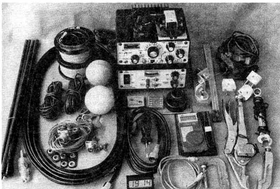
The complete W6ZH Portable Operation Package. The Worldradio Transceiver and Power Supply Unit with the 12 foot collapsible whip antenna and counterpoise wire, 20 metre dipole and feeder, clamp for the whip, mains adaptors, tools, multimeter, fishing line and tennis balls for throwing up the dipole. The complete package fits into one carry-on bag.
